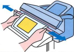
● Tensile the bag to prevent wrinkle or tunnel at sealed area.
