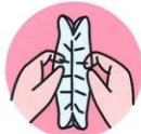
● Check the seal result condition. (Do this by pulling out the sealed area to left and right. If it peels, heating is not sufficient.)
